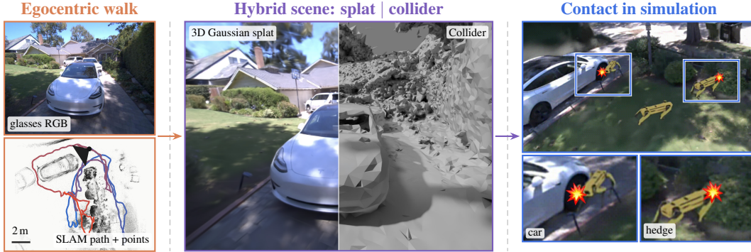
Fig. 1: Ego2Sim converts a single walk captured by head-worn glasses into a contact-enabled hybrid simulation scene : a Gaussian splat for what a robot sees and a collision mesh for contact. The Spot robots in the image (from Isaac Sim [1]) walk in a scene built from a 2.6-minute egocentric recording and make contact with the environment, as shown above.
